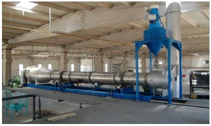
Rotary industrial dryer is an essential machine for wide ranging applications. It also acts as a calcination furnace for calcination processes.
